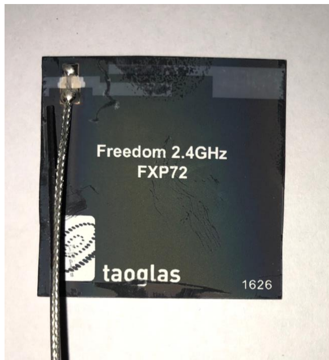
Figure 5.26: Color Gradient Seen on the 48-Hour Patch Antenna Sample.
