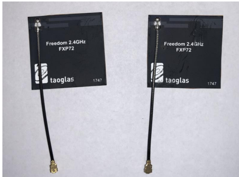
Figure 5.5: 24-Hour AO Exposed Samples that Were Placed in Positions 3 (Left) and 6 (Right).
