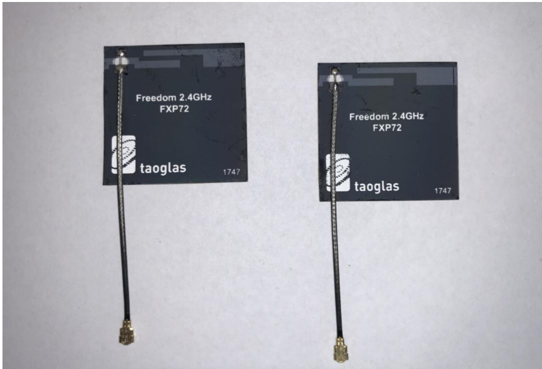
Figure 5.9: 48-Hour AO Exposed Samples that Were Placed in Positions 3 (Left) and 6 (Right).
