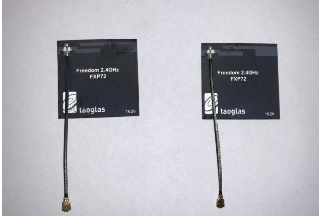
Figure 5.7: 48-Hour AO Exposed Samples that Were Placed in Positions 1 (Left) and 4 (Right).
