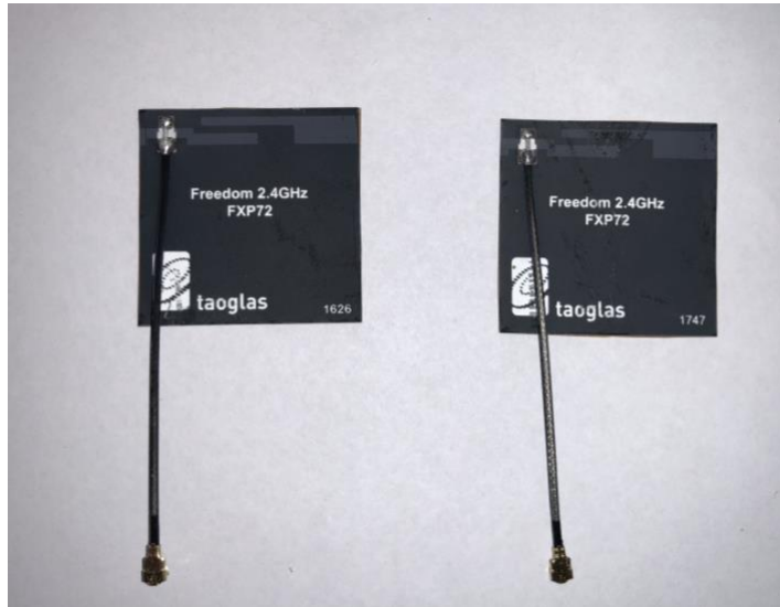
Figure 5.3: 24-Hour AO Exposed Samples that Were Placed in Positions 1 (Left) and 4 (Right).
