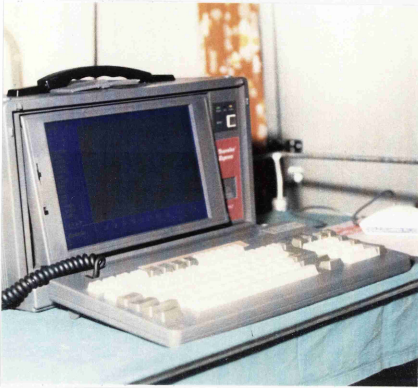
FIGURE 14. Photograph showing the computer used to measure auditory evoked responses. The screen displays the BAER and LLAER waveforms.
