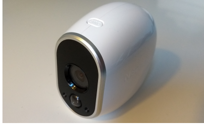
Figure 3: Wireless Netgear Arlo camera used for home recording; one for front view and one for side view.
