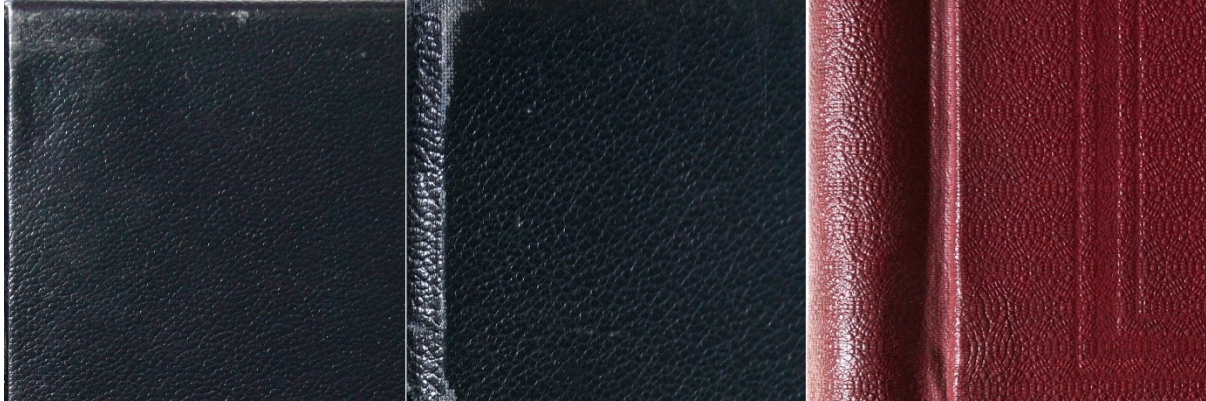
Fig.5. Nitrocellulose-coated ledger bindings of the 1920s-1930s give an idea of the appearance of automobile leathercloth. The thinner bookcloth chipped more easily (centre example). Embossing did not have to take the form of leather grain (right example). A. Brunnschweiler & Co. archive.
