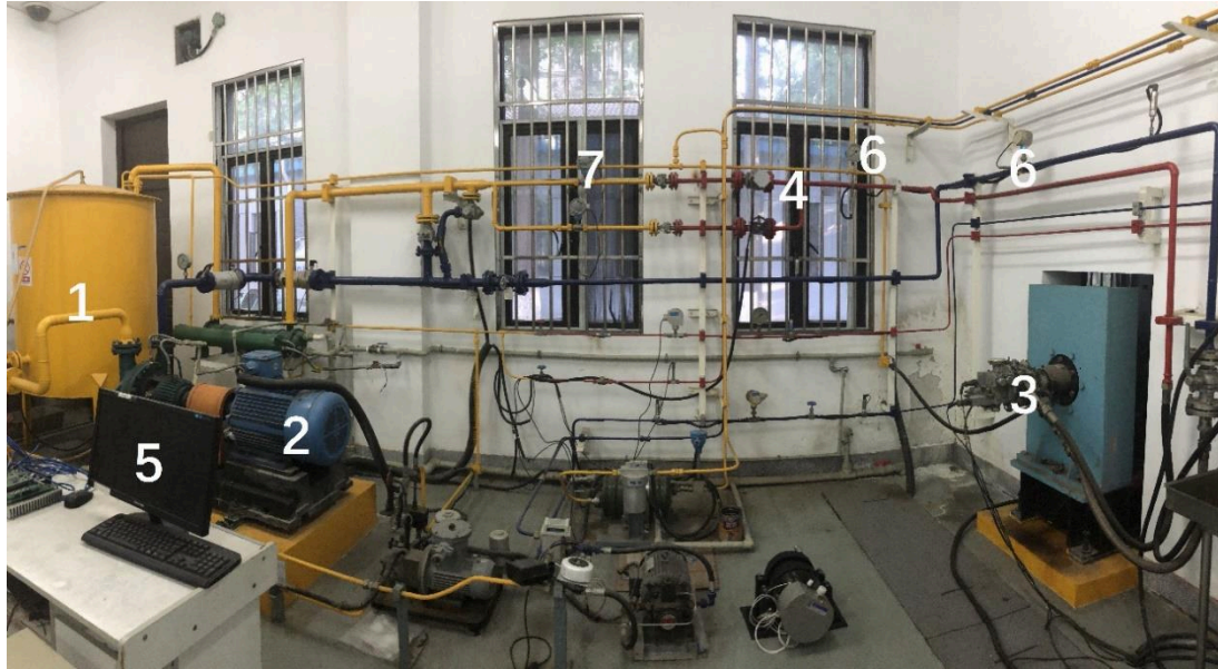
Figure 13. HIL simulation test platform. 1: fuel tank; 2: booster pump; 3: fuel control unit; 4: automatic regulating facility; 5: controller; 6: pressure transducer; 7:flow meter.
