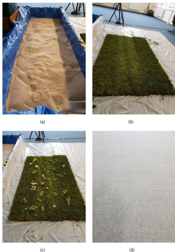
FIGURE 6. Setup of the four different test environments in the laboratory: (a) sand, (b) grass, (c) grass with foliage, (d) carpet.
