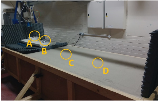
Figure 11. Laboratory sand bay with several calibration objects and a PMN-1 landmine located at the positions shown; A: 60 mm metal sphere, B: 100 mm square sided dihedral, C: 70 mm sided trihedral buried 90 mm in depth and D: 100 mm dia. x 40 mm thick PMN-1 anti-personnel landmine buried 100 mm in depth.
