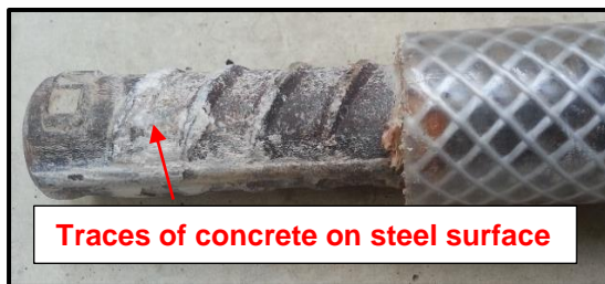
(a) Shear off concrete in cube (C-16-2.5d)
