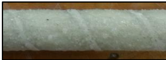
(a) Helically wrapped with sand coated surface (type A)
