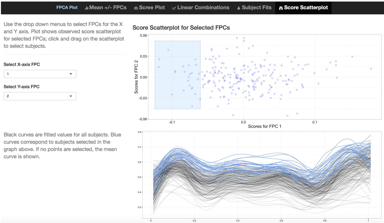
Figure 2.1: Screenshot showing tab 5 of the interactive graphics for FPCA. A scatterplot of FPC loadings \hat{c}_{ik} against \hat{c}_{ik'} is shown in the upper plot, and k and k' are selected using drop-down menus at the left. The lower plot shows fitted curves for all subjects. In the scatterplot, a subset of estimated loadings can be selected by clicking-and-dragging to create a blue box; blue curves in the plot of fitted values correspond to selected points in upper plot.
