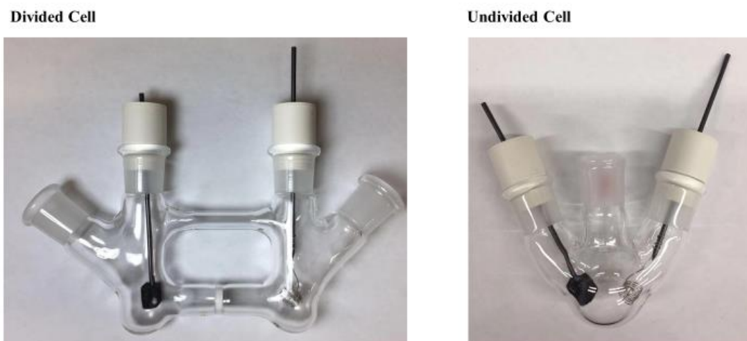
Fig. S3. Divided cell and undivided cell set up
