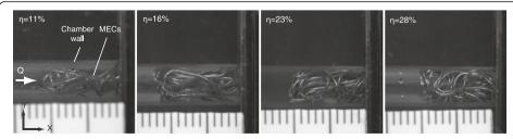
Figure 4 Packed MECs in the measuring chamber. Coil lengths of 0.28, 0.47, 0.59 and 0.71 m were randomly packed to achieve packing densities of 11, 16, 23 and 28%, respectively. Packing density (n) was calculated by dividing the volume of the coil by the cylindrical bounding volume of the coil mass.
