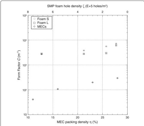
**Figure 8 Form factor of the SMP foams and MECs.** The form factor of both SMP foam types was higher than that of the MECs in all cases, and it increased for SMP foam samples with lower hole densities. The form factor of the MECs was higher for samples with higher packing density.
