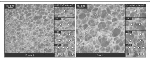
**Figure 3 SMP foams prior to mechanical reticulation and mechanical reticulation scenarios (2.5x magnification).** The solid white circles represent the holes due to mechanical reticulation (to scale). Hole density ( $\zeta$ ) was calculated by dividing the number of holes pierced by the surface area of the 3-D-printed template. The average cell size of foams S and L was 0.7E-3 and 1.1E-3 m, respectively.
