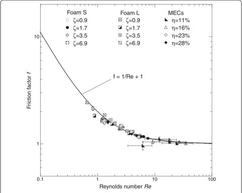
**Figure 9 Friction factor versus Reynolds number for the SMP foam samples and MECs.** The mechanical reticulation hole density ( $\zeta$ ) has units E + 5 holes/m². The friction factors and Reynolds numbers for both SMP foam types and for the MECs collapse onto the relationship specified by Equation 3 for Reynolds numbers ranging approximately from 1 to 35. The friction factors of all SMP foam samples were higher than those of the MECs.
