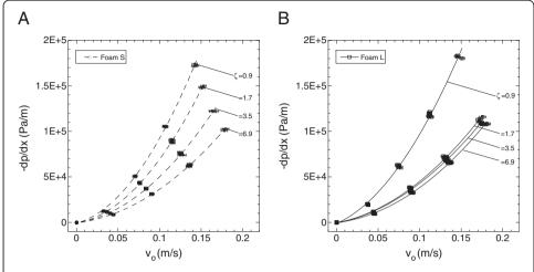
Figure 5 Pressure gradient versus Darcy velocity of reticulated SMP foams S (A) and L (B). The mechanical reticulation hole density ( $\zeta$ ) has units E + 5 holes/m<sup>2</sup>. As the hole density increases, the pressure gradient across the samples also decreases for both SMP foam types.
