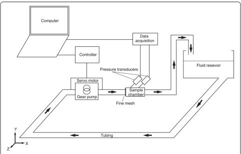
**Figure 1 Flow system constructed to measure the pressure gradient along the SMP foam and MEC samples.** The pressure gradient was measured utilizing two high accuracy pressure transducers, and the flow rate was measured by hand with a graduated cylinder and a digital stop watch. A fine mesh (stainless steel 316, 0.1E-3 m wire diameter, 4E-7 m<sup>2</sup> squares) was installed at the inlet of each sample chamber to homogenize the incoming flow.
