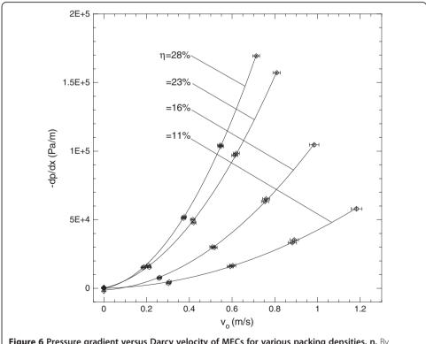
**Figure 6** Pressure gradient versus Darcy velocity of MECs for various packing densities,  $\eta$ . By increasing the packing density of the MECs, the pressure gradient across the samples also increases.
