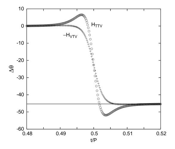
FIG. 1: The rotation of the Laplace-Runge-Lenz vector due to second order error Hamiltonian  $-H_{VTV}$  and  $H_{TTV}$  in algorithms I and II. Each algorithm rotates the LRL vector differently in time, but by exactly the same amount after one period. Most of the rotation takes place near the mid period. The solid line gives the theoretical value of -45.33318.
