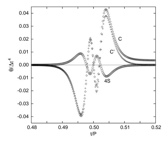
FIG. 4: The rotation of the Laplace-Runge-Lenz vector for three fourth-order integrators: algorithm C, algorithm C' with added gradient term to force the rotation angle back to zero, and the true symplectic corrector algorithm 4S. As with most integrators, algorithm C's precession error does not return to zero.
