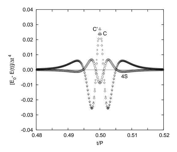
FIG. 5: The energy error functions of algorithms C, C  $^{\prime}$  and 4S. Algorithm 4S's maximium error is three times smaller than that of C.
