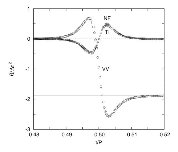
FIG. 3: The rotation of the Laplace-Runge-Lenz vector for three second-order symplectic algorithms: velocity-Verlet (VV), Takahashi-Imada (TI) and the non-forward corrector algorithm (NF). The solid line gives the theoretical rotation value of the VV algorithm:  $\Delta\theta_{TTV}/24 = -1.8888$ .
