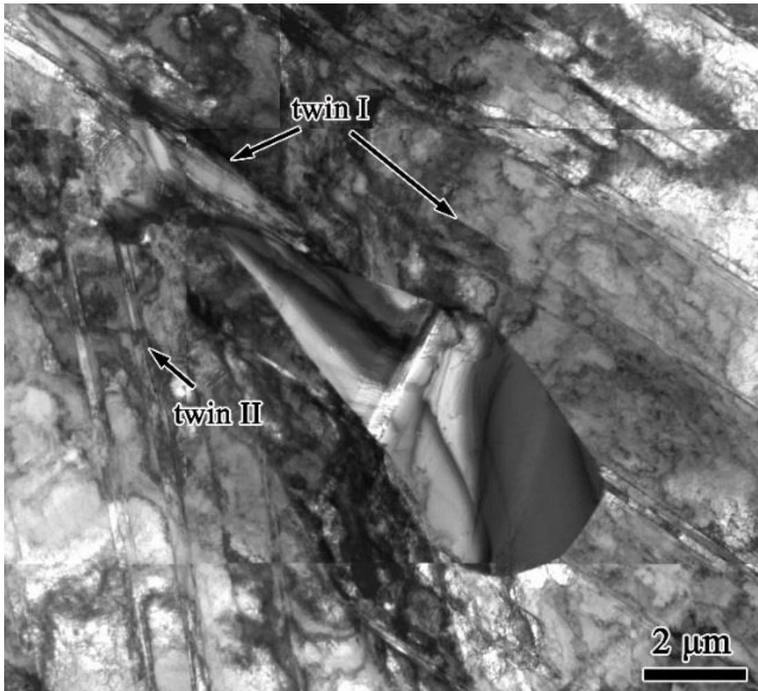
Figure 24 Bright field TEM image collage of the 316 SS specimen deformed to 30% tensile strain and annealed at 900°C for 1 hr. The recrystallization starts from the intersection of two different twin variants.
