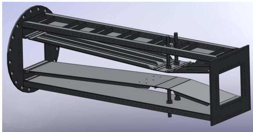
Figure C-172. Contour of old diffuser: nuts on threaded rods for throat adjustment
