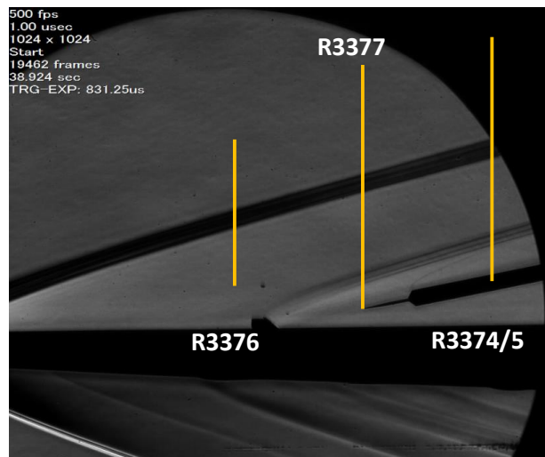
Figure 68. Approximate hot-wire probe paths (vertical yellow lines) for characterization of the leading-edge shock, overlaid on a schlieren image.
