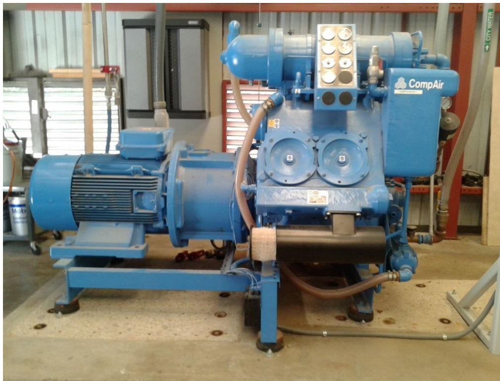
Figure 43. CompAir Reavell 5442 compressors
