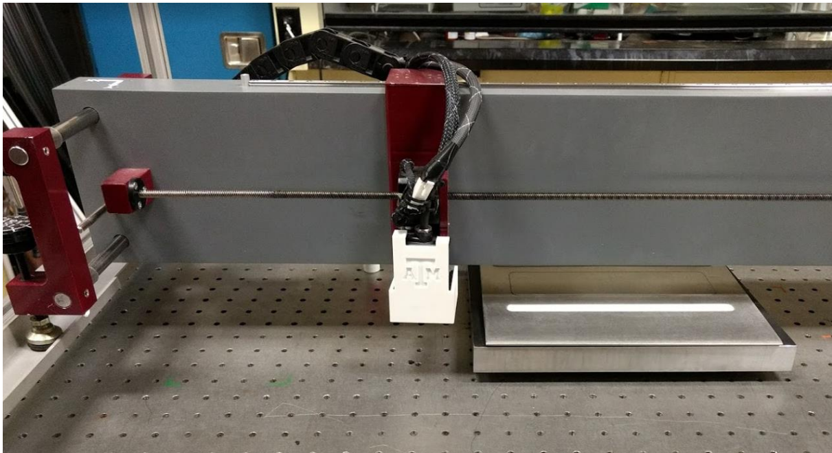
Figure E-178. Setup of laser profilometer and model for leading-edge scans
