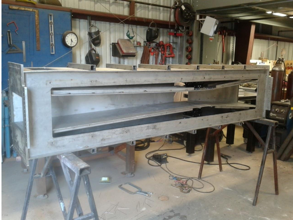
Figure C-176. Fabrication of stainless diffuser
