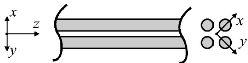
FIG. 1. The geometry of the ion trap and the coordinate system used in this simulation. Trap electrodes extend infinitely along the z axis. The x and y axes point toward the trap electrodes.
