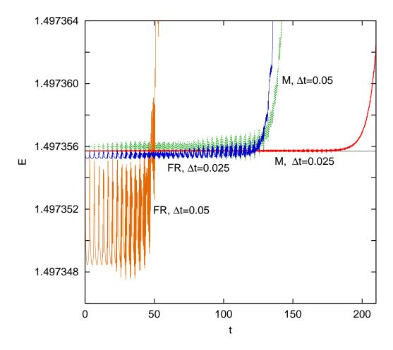
FIG. 2: (Color online) A magnified view of the fluctuation in the total energy of two fourth-order algorithms FR and M at two time-step sizes.
