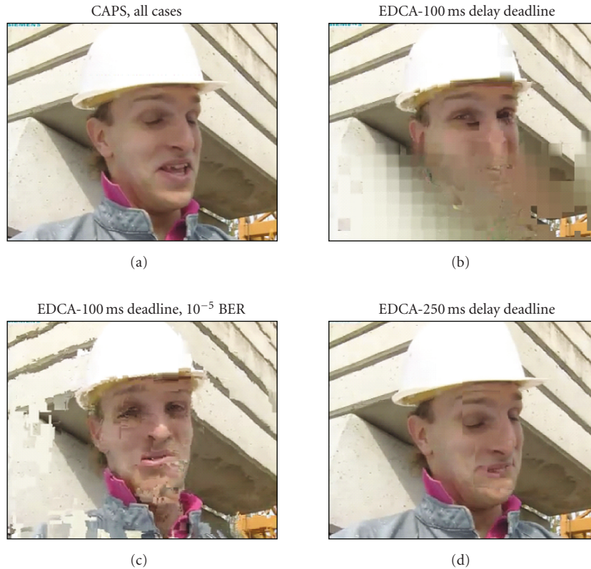
FIGURE 7: Snapshots of foreman video, transmitted over a WLAN with delay deadlines of 100 and 250 microseconds.
