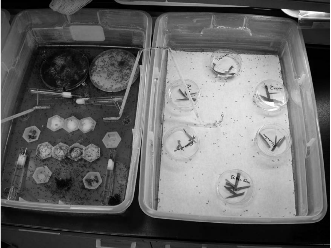
Fig. 1. Procedure for exposing test grasses to foraging ants from a lab colony of red imported fire ants. Fire ant colony is positioned next to the test arenas with the grass selections. Ants can pass through a glass travel tubes from the colony to the test arena to forage on selected grasses.
