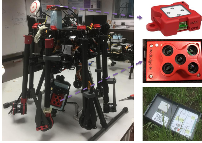
Figure 3: Image acquisition by an UAV-Camera system: DJI S1000 Octocopter (left), Downwelling light sensor (top-right), RedEdge camera (middle-right) and panel for reflectance calibration (bottom-right).
