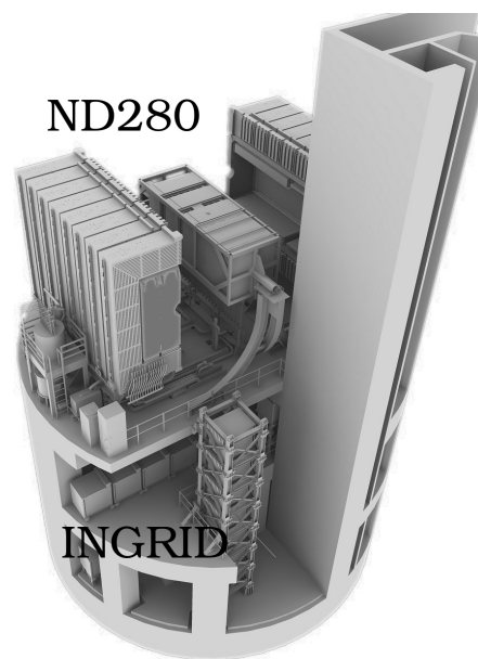
Figure 3.2.: The suite of near-detectors at 280 m from the target, showing ND280 and INGRID
