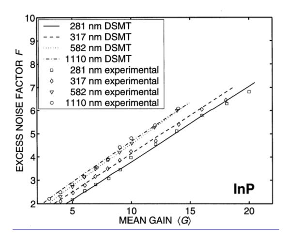
**Fig. 6.** Comparison of the DSMT-predicted and the experimental excess noise factor *Fversus* mean gain  $\langle G \rangle$  for four thin InP APDs with different multiplication-region widths. Symbols represent experimental data and curves represent predictions using the DSMT.
