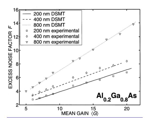
**Fig. 9.** Comparison of the DSMT-predicted and the experimental excess noise factor *Fversus* mean gain  $\langle G \rangle$  for three thin Al0.2Ga0.8As APDs with different multiplication-region widths. Symbols represent experimental data and curves represent predictions using the DSMT. Though the data are identical to those presented in [4], an improved fitting procedure has been used.
