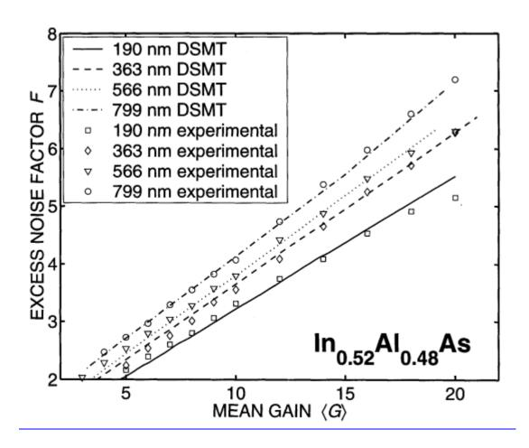
**Fig. 7.** Comparison of the DSMT-predicted and the experimental excess noise factor *Fversus* mean gain  $\langle G \rangle$  for four thin In0.52Al0.48As APDs with different multiplication-region widths. Symbols represent experimental data and curves represent predictions using the DSMT.
