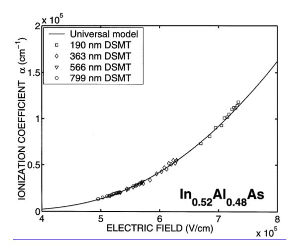
**Fig. 4.** Electron ionization coefficient ( $\alpha$ ) of In0.52Al0.48As as a function of the electric field. Symbols represent calculated values of the ionization coefficients of capable carriers for four thin In0.52Al0.48As APDs (thickness indicated in inset), using the DSMT. The solid curve represents the universal exponential model.
