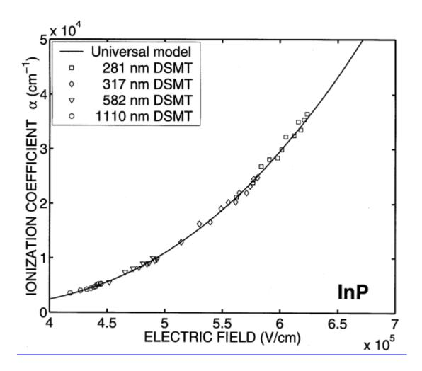
**Fig. 2.** Electron ionization coefficient ( $\alpha$ ) of InP as a function of the electric field. Symbols represent calculated values of the ionization coefficients of enabled carriers for four thin InP APDs (thickness indicated in inset), using the DSMT. The solid curve represents the universal exponential model.
