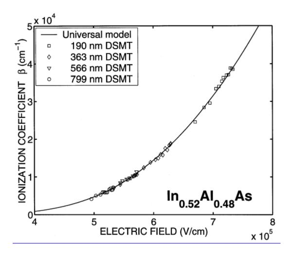
**Fig. 5.** Hole ionization coefficient ( $\theta$ ) of In0.52Al0.48As as a function of the electric field. Plot symbols are the same as in Fig. 4.
