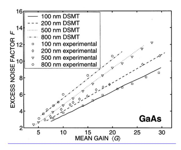
**Fig. 8.** Comparison of the DSMT-predicted and the experimental excess noise factor *Fversus* mean gain  $\langle G \rangle$  for four thin GaAs APDs with different multiplication-region widths. Symbols represent experimental data and curves represent predictions using the DSMT. Though the data are identical to those presented in [4], an improved fitting procedure has been used.
