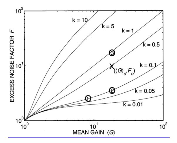
**Fig. 1.** General characteristics of the excess noise factor (F) versus the mean gain ( $\langle G \rangle$ ) parameterized by the hole-to-electron ionization ratio k, according to the conventional McIntyre theory [7]. The encircled points 1, 2, and 3 are samples of the ( $\langle G \rangle$ ,F) values generated in the process of finding the ionization coefficients of enabled carriers using the dead-space theory.
