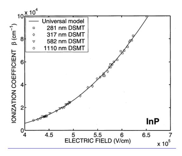
**Fig. 3.** Hole ionization coefficient (*6*) of InP as a function of the electric field. Plot symbols are the same as in Fig. 2.
