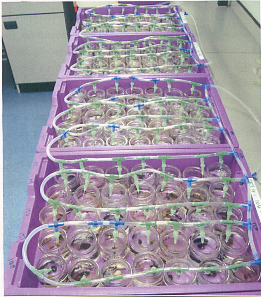
Figure 4.2: Photograph of the feeding trials (i.e. the experimental system used for quantifying leaf consumption rate by individuals of different shredder species) (see Section 4.2.2.2.).
