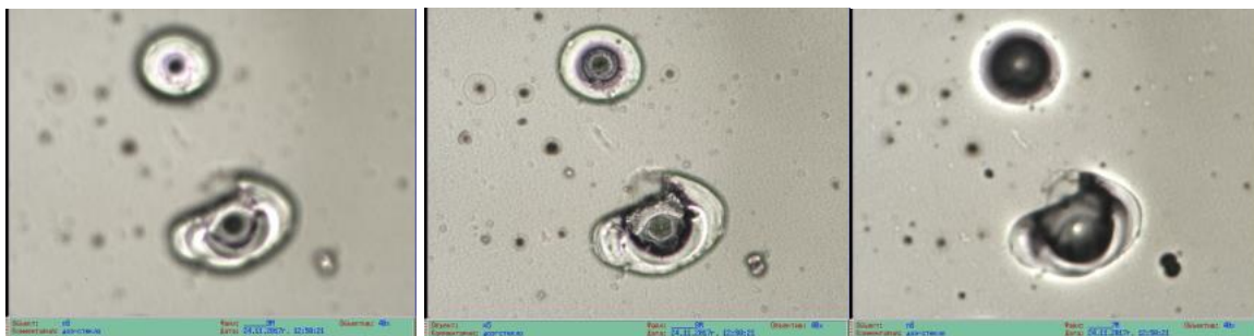
Figure 8. Diffraction of light on microspheres formed in glass with a protective film when exposed to laser radiation
