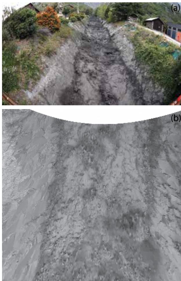
Figure 3. (a) Original footage of a flash flood in the St-Julien torrent acquired by a storm chaser equipped with Canon EOS 5D mark II camera. The direction of flow is from the top of the frame, moving towards the bottom of the image; (b) Orthorectified and geometrically stable image with the field of view clipped to the lower 50% of the image. The direction of flow is from the bottom of the frame, moving towards the top of the image.
