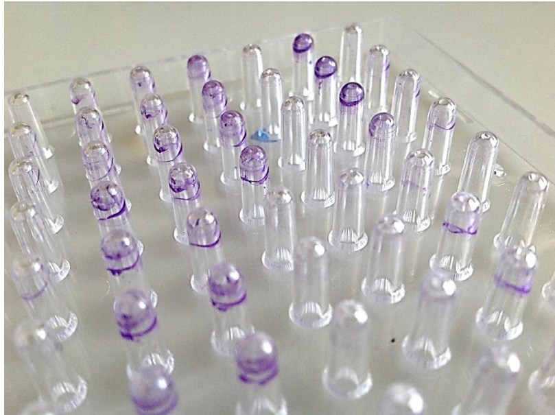
Figure 27: Crystal violet stained biofilm coating the surface of a "Calgary peg" plate lid prior to the elution of the stain into the 96 well plate using absolute ethanol. Varying levels of biofilm retention can be measured using a colorimeter to determine the differing effects of biocide on the biofilm matrix of different species.
