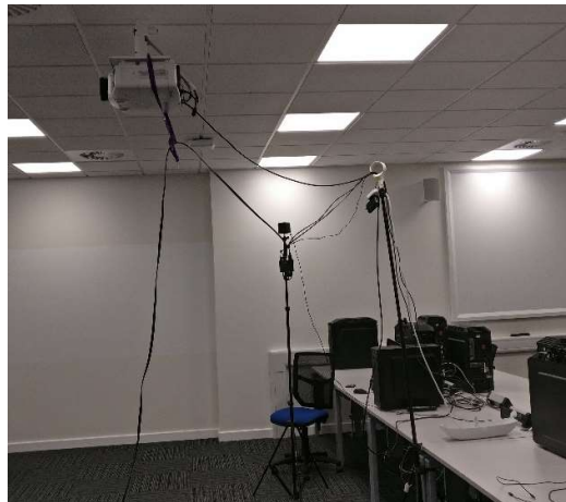
Figure 5: Lab setup used to suspend the cable above the user's head, the project is near the centre of the play area used by participants.
