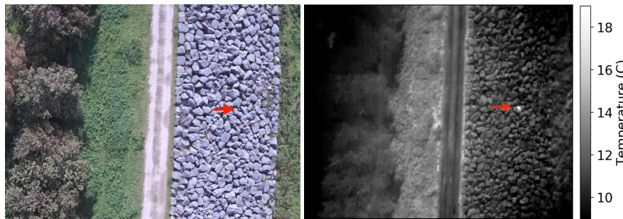
Figure 2. RGB (left) and TIR (right) images taken from the drone showing the same scene for one of the search and rescue scenarios performed. The volunteer hiding in rocks is very difficult to discern in the RGB image but appears as a bright source in the TIR image (indicated with an arrow).
