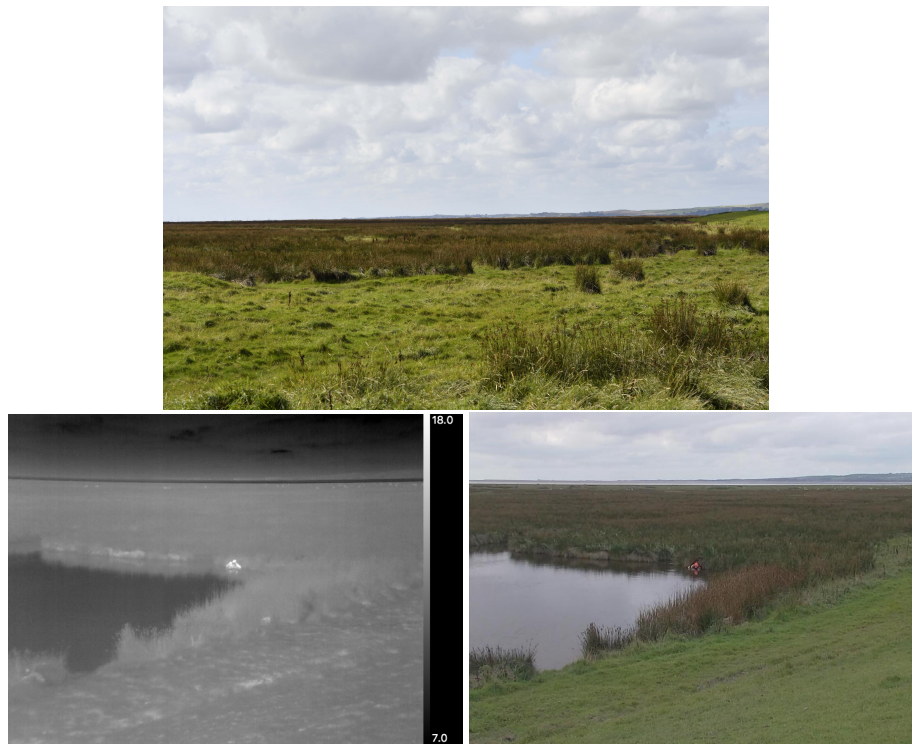
Figure 1. Example images of the terrain at Morecambe Bay when viewed from the ground, illustrating the challenges of finding people in need of rescue on foot. The bottom row shows the same scene viewed with a TIR camera ( left ) and RGB camera ( right ), where a volunteer in the water is in the middle of the field of view. The colour bar for the left-hand figure indicates the measured temperature in °C.
