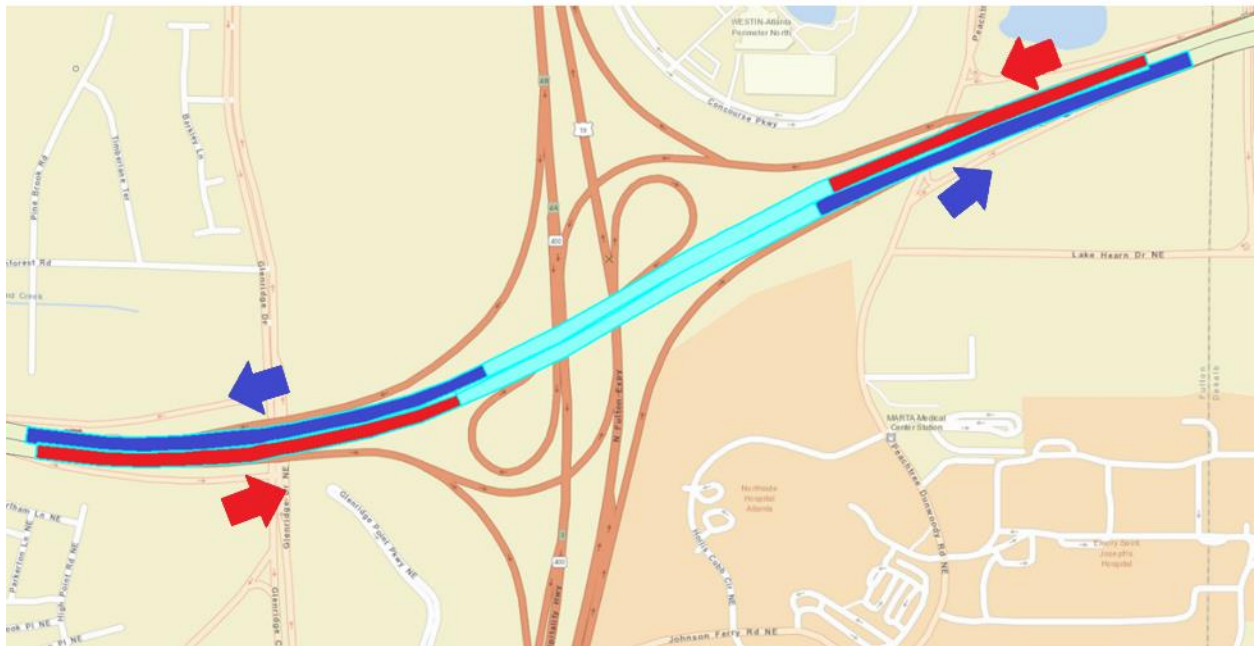
Figure 17. Classification of road segment based on position in interchange.
