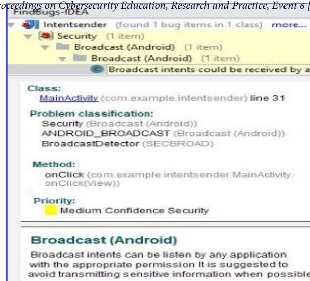
Figure 3: Broadcast intent detected by FindSecurityBugs
