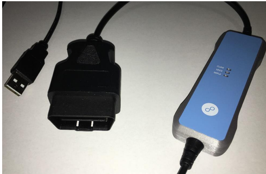
Figure 1: The Korlan USB2CAN adapter ($70 USD) connects a laptop or desktop computer to the OBD-II port in most cars and trucks sold in the US since 1996.
