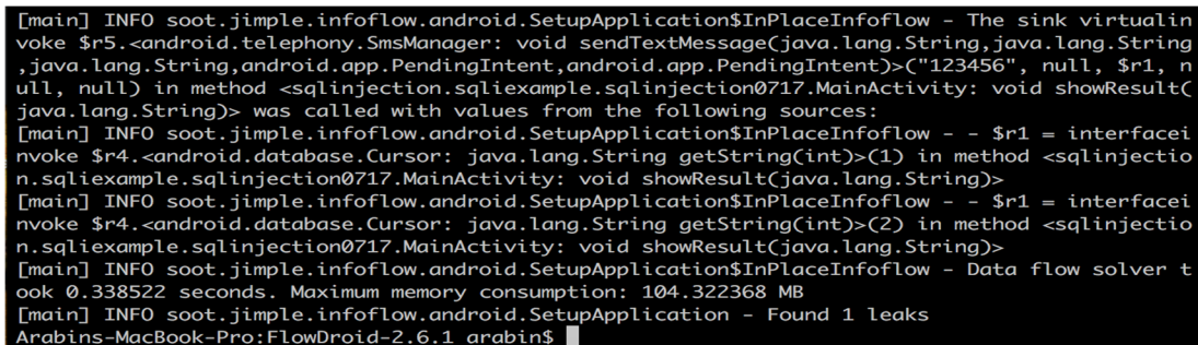
Figure 13. Data flow analysis by FlowDroid
