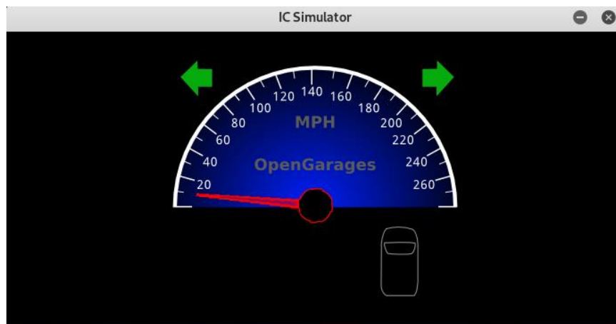
Figure 7: We have successfully reverse engineered the CAN ID and data values needed to hack the turn signals, gaining full control of both turn signals in the IC Simulator.
