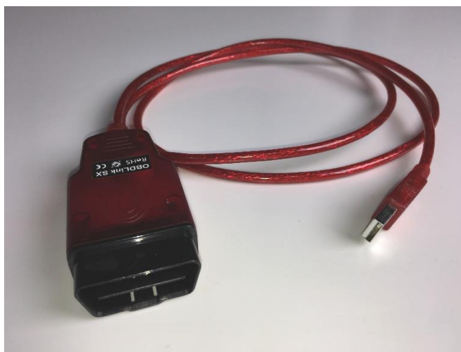
Figure 8: You can purchase a USB to OBD-II adapter cable to connect your computer to almost any post-1996 automobile's on-board-diagnostic (OBD) port, for just around $20-30USD online.
