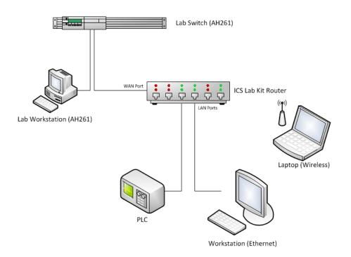
Figure 3. The Defensive Security Equipment Setting
