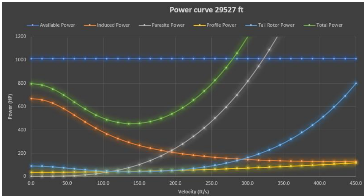
Figure 5-3. Forward flight at 29527 ft.
