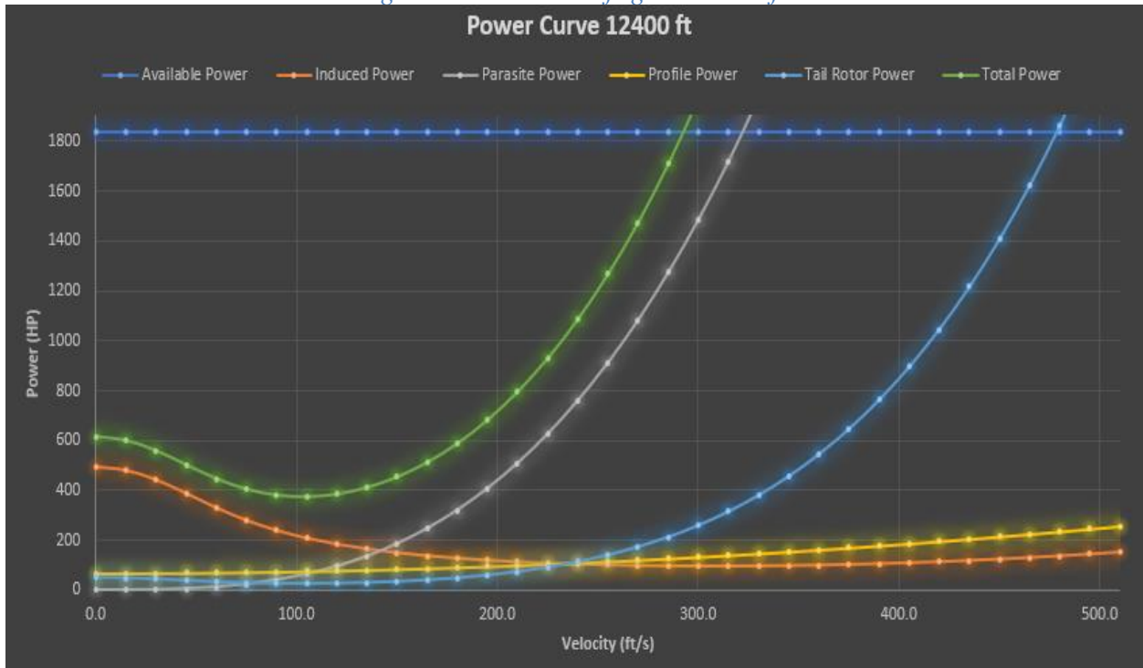
Figure 5-2. Forward flight at 12400 ft.
