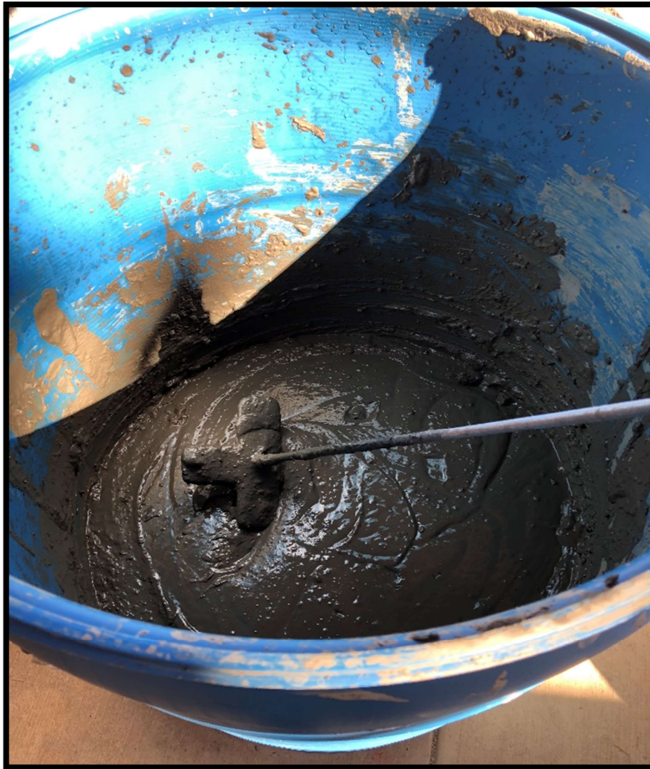
Figure 3.8: “Parent” slurry being mixed with high speed electric mixer in 50-gallon drum barrel.
