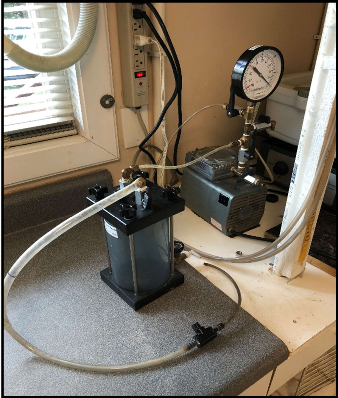
Figure 3.7: Vacuum pump set-up for decanting free water after testing period is over.
