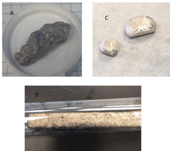
Fig. 1 Synthesized schreibersite samples. (A) Vesicular schreibersite obtained by rapid cooling. (B) Schreibersite sample obtained by slow cooling. (C) Dense schreibersite samples obtained when specimen were heated to the eutectic melting point after 235 h. Samples are 1 cm in width, defined by the width of the alumina crucible.
