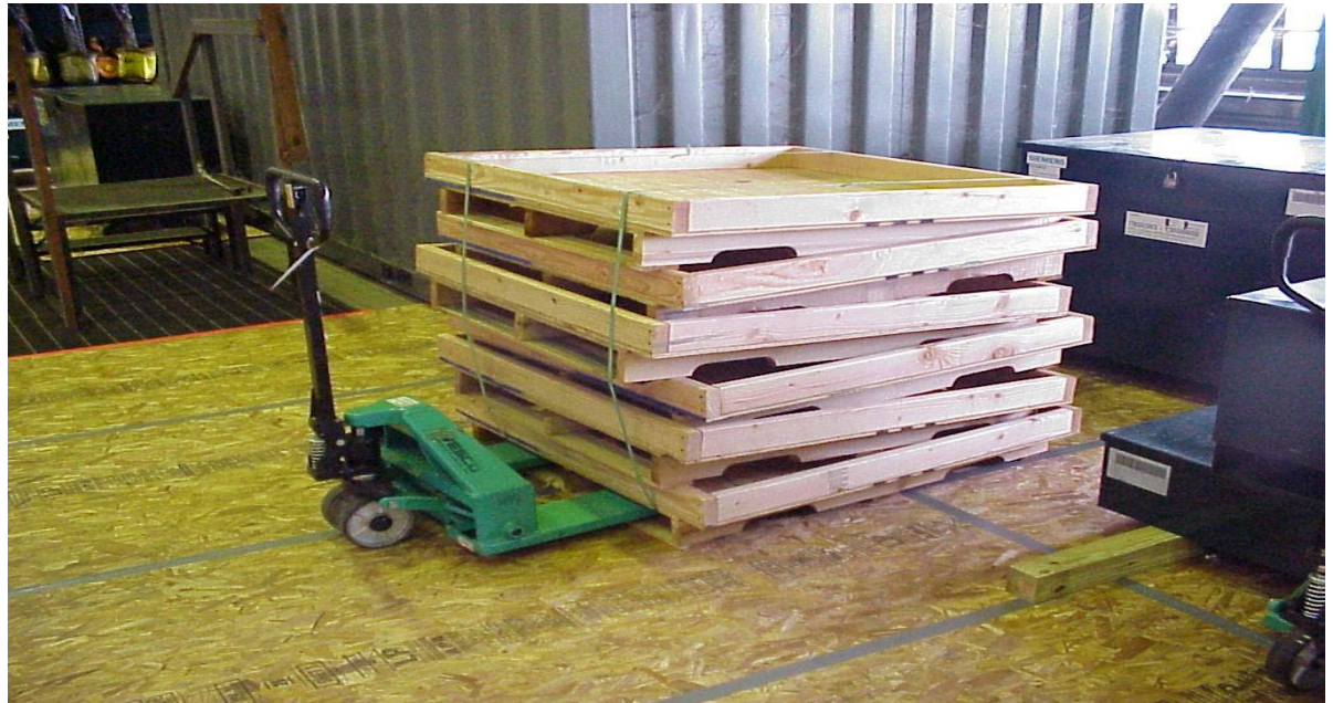
Figure 46: Custom-built Pallet (48" x 48" x 5" with 1/2" Plywood Top, 2" x 4"
