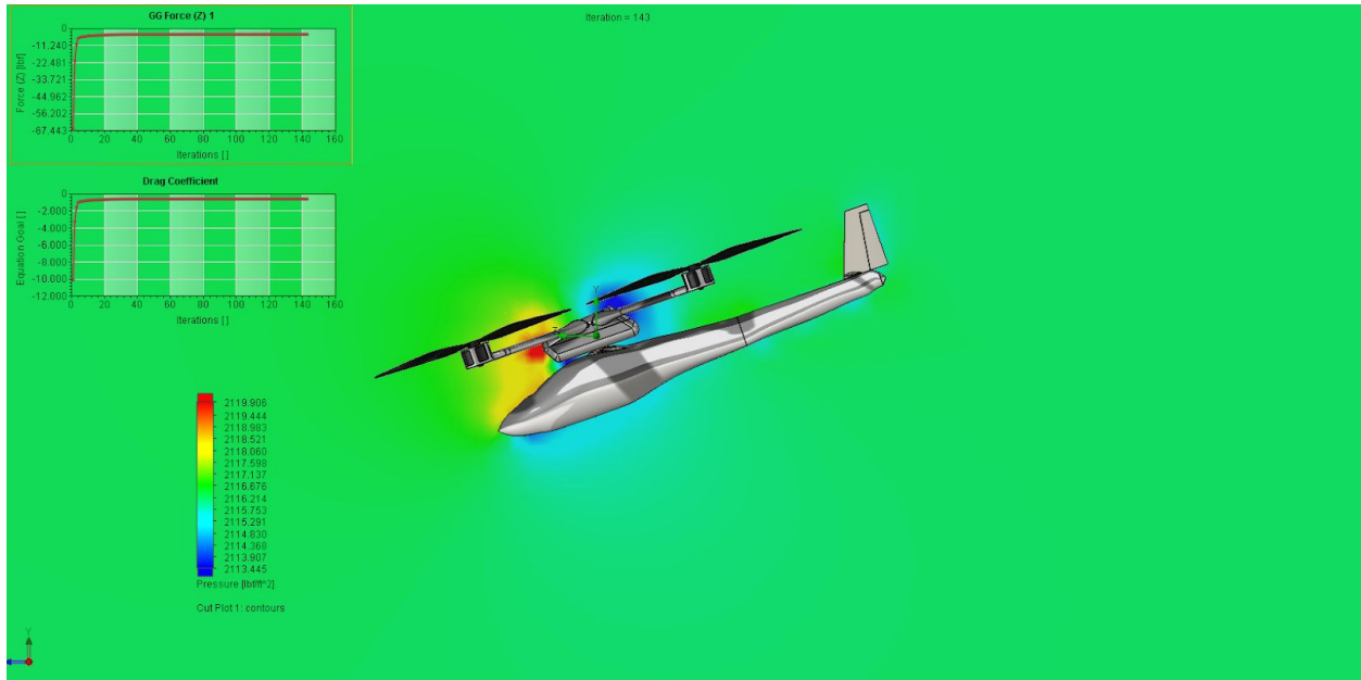
Figure 31. Pitched UAS Pressure Contour
