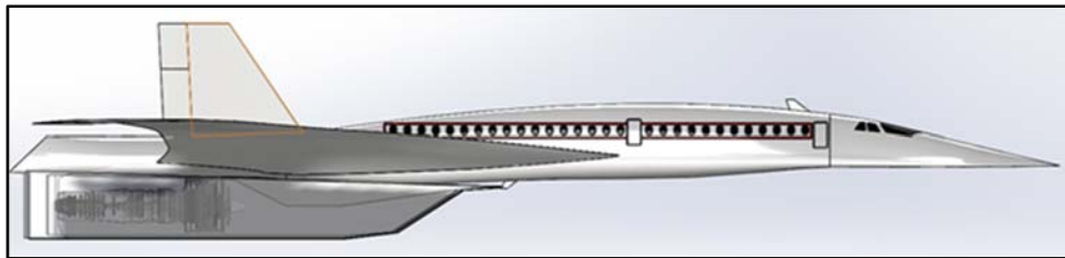
Figure 41: Design concept with engine location configuration for Orientation 2 (two engines below fuselage)
