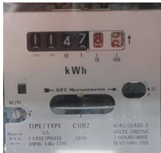
Figure 6: Electricity meter with kWh output (Zietsman, 2015)
