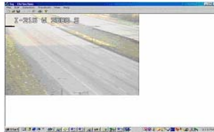
Figure 5: Background Image developed from 100 captured frames
