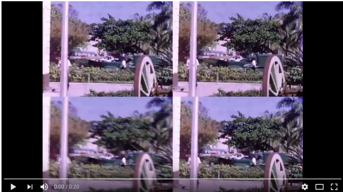
Top Left: 12 fps film with every-other frame repeated to create 24 fps. Top Right: 12 fps conformed to 24 fps. Bottom Left: 12 fps converted to 24 using Adobe's frame blending. Bottom Right: 12 fps to 24 fps using Adobe's pixel motion interpolation. (00:20)
