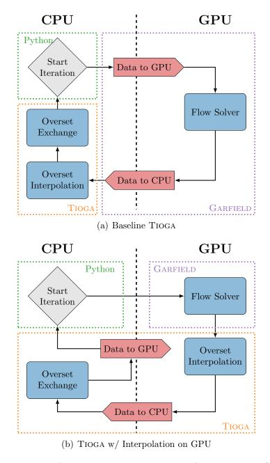
Figure 2.21: Flowchart of routines showing location of data: on the CPU or on the GPU. Performing interpolation on the GPU drastically reduces data transfer to the CPU.
