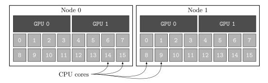
Figure 2.23: Cluster node topology with 2 GPUs and 16 CPU cores per node.
