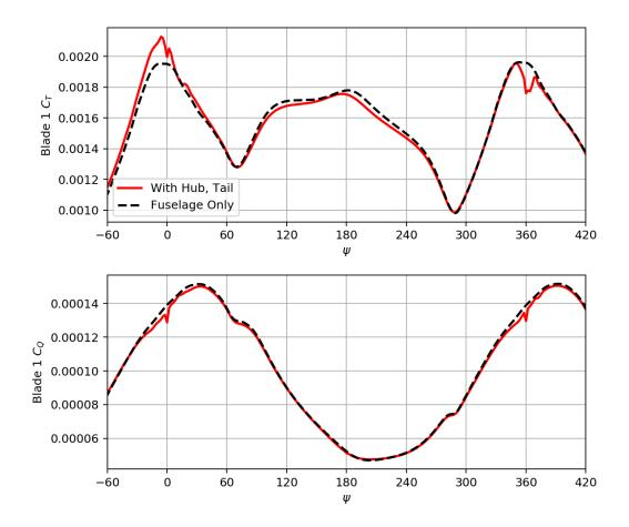
Figure 4.9: Comparison of Blade 1 Loads with and without hub and tail rotor.
