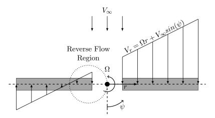
Figure 1.3: Illustration of aerodynamic variation across a rotor blade in forward flight. A reverse-flow region develops on the retreating side.
