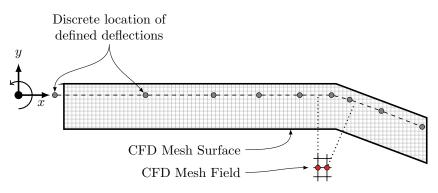
Figure 2.17: Control points along blade where deflections are defined. Distances to CFD coordinates may be discontinuous.
