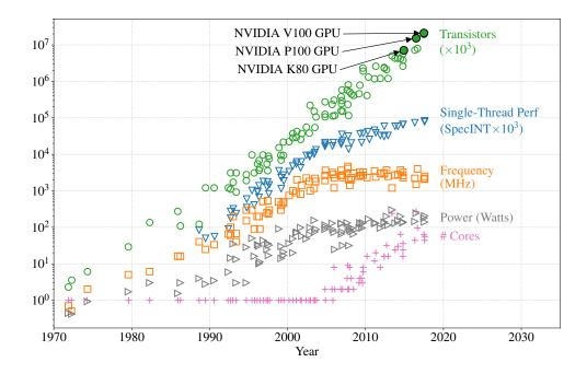
Figure 1.10: 45 years of micro-processor data with the transistor counts of three NVIDIA GPUs highlighted. Original data up to the year 2010 collected by M. Horowitz, F. Labonte, O. Shacham, K. Olukotun, L. Hammond, and C. Batten. New data collected for 2010-2015 by K. Rupp [2].
