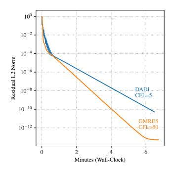
Figure 3.15: Wall-clock time comparison of convergence with DADI and GMRES methods.
