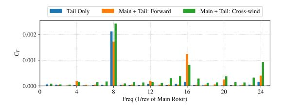
Figure 4.22: Tail rotor thrust coefficient frequencies
