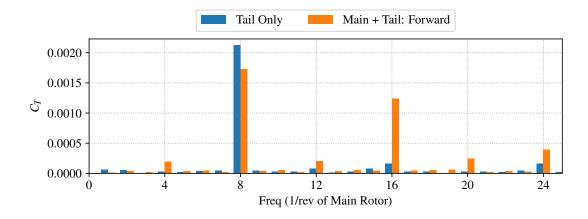
Figure 4.19: Tail rotor thrust coefficient frequencies
