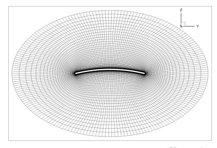
Figure 5.4: Blade cross-section showing cambered, 2% thick flat plate.
