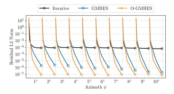
Figure 5.8: Iteration convergence after  $t^*$ :  $\Delta \psi = 1^\circ$ . Dual-time CFL is  $\infty$  for GMRES and O-GMRES methods and 100 for the Iterative method.
