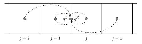
Figure 2.2: MUSCL 3-point stencil for left and right primitive variables  $q_L$  and  $q_R$ .
