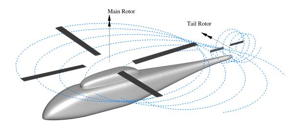
Figure 1.1: Illustration of the wake of a single-main-rotor helicopter. The tip vortices, shown as dotted lines, may interact with the fuselage and tail rotor.
