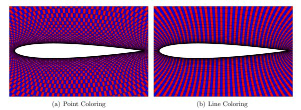
Figure 2.5: Illustration of red-black coloring.
