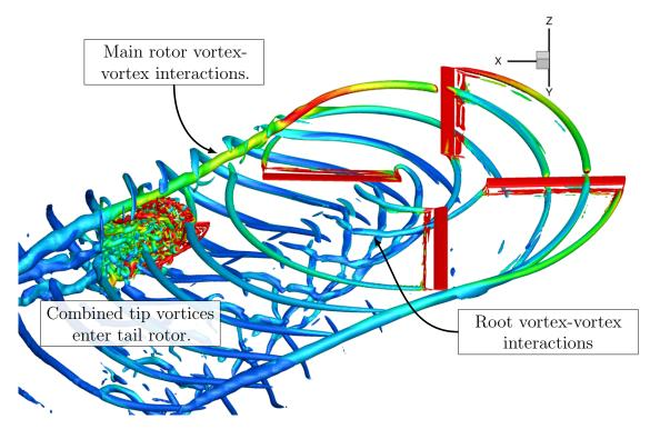
Figure 4.20: Main and tail rotor Q-criterion (Q = 0.0008) solution in cross-wind flight.
