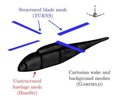
Figure 4.2: Fuselage and blade surfaces for CFD domain.
