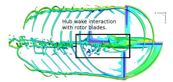
Figure 4.8: Iso-surfaces of vorticity: blade 1 near  $\psi = 0$  passes through wake of hub.
