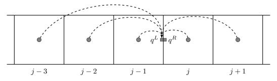
Figure 2.3: WENO 5-point stencil for left and right primitive variables  $q_L$  and  $q_R$ .
