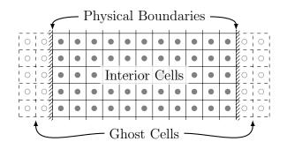
Figure 2.6: Full domain consisting of interior cells, ghost, cells, and boundaries.
