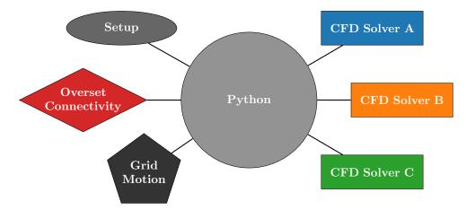
Figure 2.22: Modules for CFD framework.
