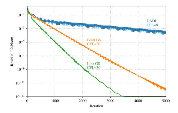
Figure 3.11: Per-Iteration comparison of convergence with DADI and two Gauss–Seidel methods.
