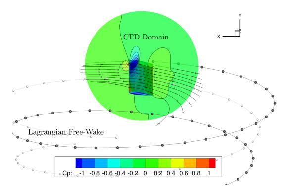
Figure 1.6: Hybrid Navier–Stokes + free-wake model of a rotor in hover. The CFD domain is near the blade and Lagrangian free-wake models the wake below the rotor.
