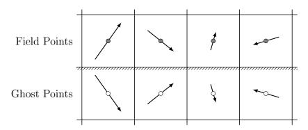
Figure 2.10: Inviscid wall boundary condition: mirrored velocities.
