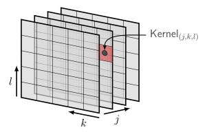
Figure 2.13: One CUDA Kernel used per (j, k, l) cell ("Point-Parallel").
