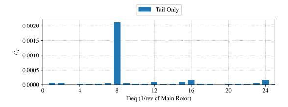
Figure 4.16: Tail rotor mean-removed thrust coefficient frequencies.
