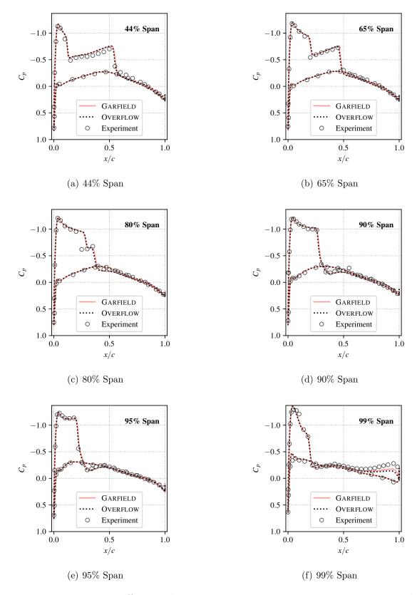
Figure 3.2: Pressure coefficient solution at six wing sections comparing experimental, GARFIELD, and OVERFLOW results.
