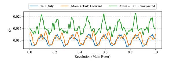
Figure 4.21: Tail rotor thrust coefficient
