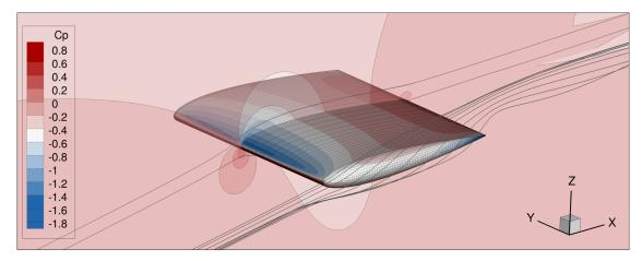
Figure 3.10: Short, inviscid NACA0012 wing used as a representative mesh for convergence analysis.
