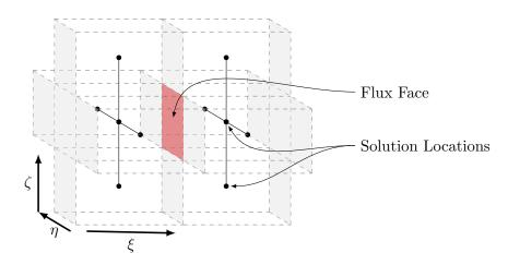
Figure 2.4: Viscous flux stencil for finite-difference relations.
