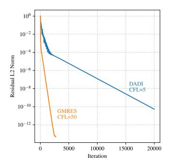
Figure 3.14: Per-Iteration comparison of convergence with DADI and GMRES methods.
