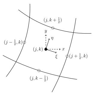
Figure 2.1: Cell-centered, curvilinear mesh for cell (j, k) with computational coordinate directions.
