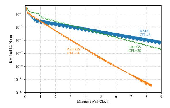
Figure 3.12: Wall-clock time comparison of convergence with DADI and two Gauss–Seidel methods.
