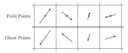
Figure 2.11: Viscous wall boundary condition: negative velocities.
