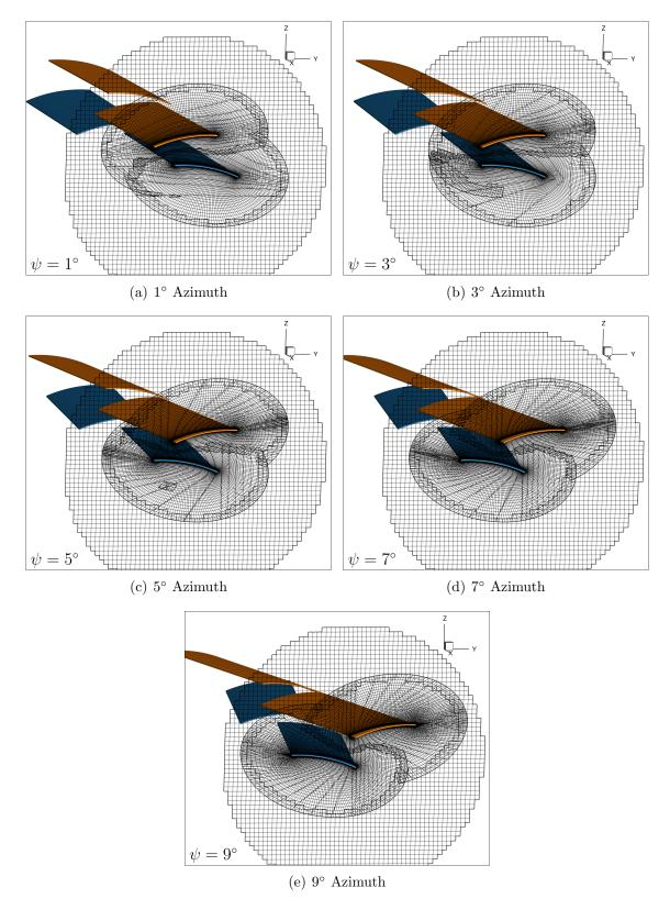
Figure 5.7: Grid and slice location at five azimuths.
