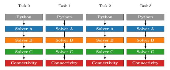
Figure 1.8: Example distribution of tasks suitable for a CPU-only CFD framework. Each solver uses all available MPI tasks.
