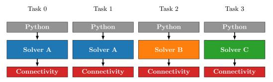
Figure 2.25: Example distribution of tasks suitable for a CPU-GPU framework. Different tasks assigned different solvers.
