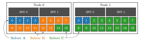
Figure 2.26: Example distribution of resources for a 3-Solver framework where Solver A is GPU-accelerated.
