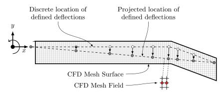
Figure 2.18: Use of projected control points results in continuous distances to CFD coordinates.
