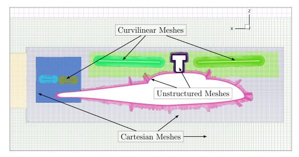
Figure 1.7: Overset CFD mesh system: unstructured and structured meshes used together.
