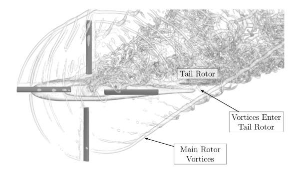
Figure 1.4: Rotor wake for a single-main-rotor in cross-wind flight. Main rotor vortices convect into the path of the tail rotor, possibly resulting in a dangerous flight condition.
