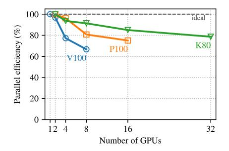
Figure 3.6: Strong scaling efficiency of Kepler (cases 1-5), Pascal (cases 7-10) and Volta (cases 11-13,16) GPUs.
