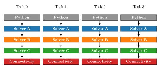
Figure 2.24: Example distribution of tasks suitable for a CPU-only CFD framework. Each solver uses all available MPI tasks.
