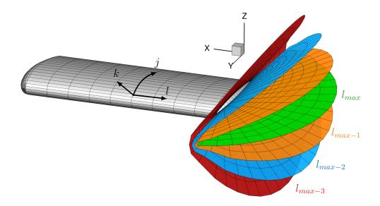
Figure 2.9: Wake boundary condition at root and tip of blade or wing meshes.
