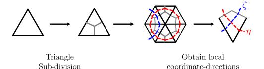
Figure 2.16: General procedure in 2D for obtaining Hamiltonian paths used as local coordinate directions.
