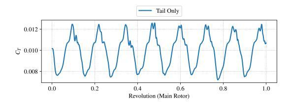
Figure 4.15: Tail rotor thrust coefficient.
