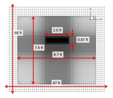
Figure 5.5: Overset grid system for the laminar coaxial rotors.
