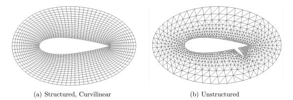
Figure 1.5: Examples of a structured, curvilinear mesh and an unstructured mesh for two airfoils.
