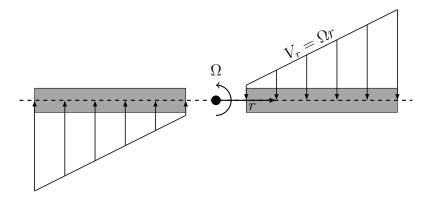
Figure 1.2: Illustration of aerodynamic variation across a rotor blade in hover.
