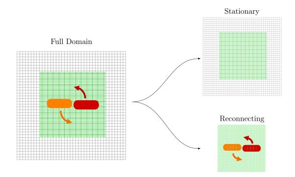
Figure 2.19: Grouping of stationary meshes and reconnecting separately so that only the "reconnecting" group reconnects every timestep.
