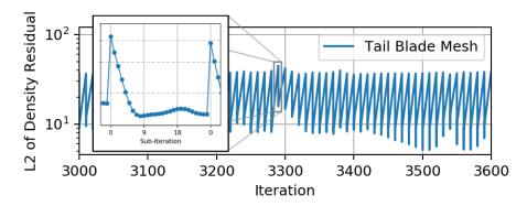
Figure 4.12: Tail-rotor sub-iterative convergence (volume-scaled L2 norm of Density residual).
