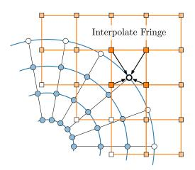
Figure 2.20: Illustration of the interpolation step for two overset grids with fringe points as hollow symbols, field points as solid symbols.
