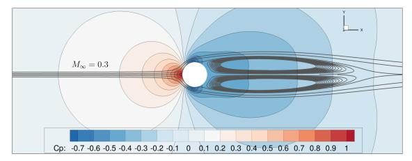
Figure 3.13: Pressure solution over a laminar cylinder with  $M_{\infty} = 0.3$  and Re = 100.
