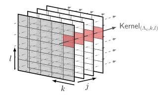
Figure 2.14: In J-direction, one CUDA Kernel used per cell eigenvalue in a k-l plane.
