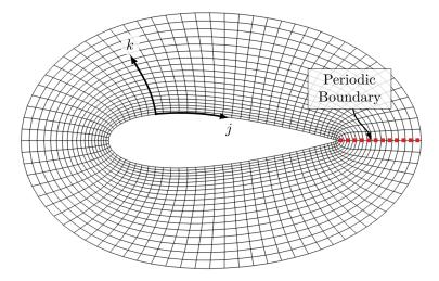
Figure 2.8: O-Mesh curvilinear coordinates result in a periodic boundary in the wrap-around direction.
