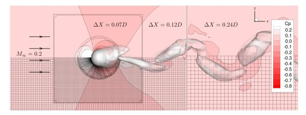
Figure 5.1: Iso-surface of Q-criterion (0.0001) with contours of Pressure Coefficient at time  $t^*$ .
