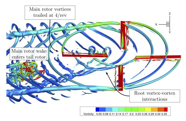
Figure 4.17: Main and tail rotor Q-criterion (Q = 0.0008) solution in forward flight
