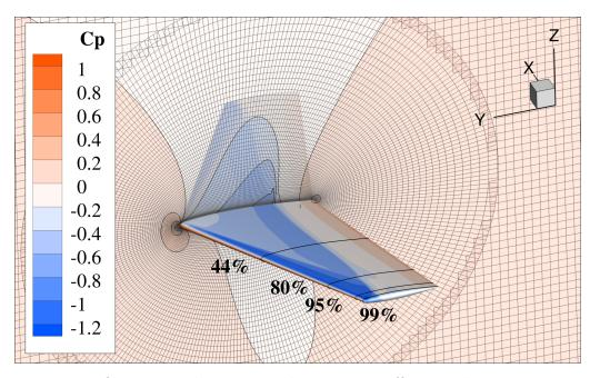
Figure 3.1: Overset mesh system and pressure coefficient solution contours.
