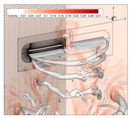
Figure 5.6: Iso-surface of Q-criterion(0.003) with contours of vorticity.
