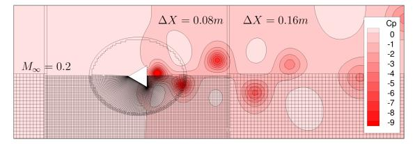
Figure 3.18: Solution and grid system for time-accurate wedge
