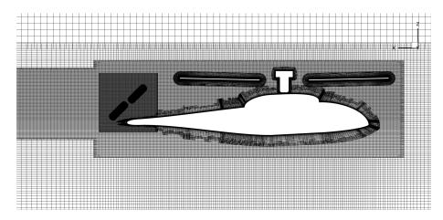
Figure 4.7: Mesh System for full configuration.
