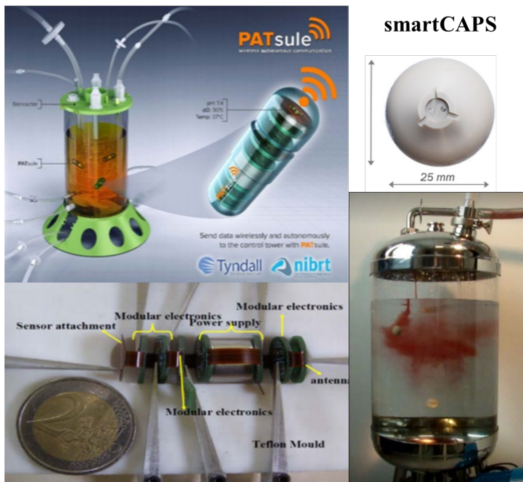
Figure 1-9. Commercial bioprocessing capsules for in situ monitoring within bioreactors. (Left) Illustration of PATsule a wireless bioprocess monitoring node derived from ingestible capsule technology [29], [104]. (Right) Illustration of smartCAPS module, and demonstration of mixing within agitated bioreactor (smartINST) [103].
