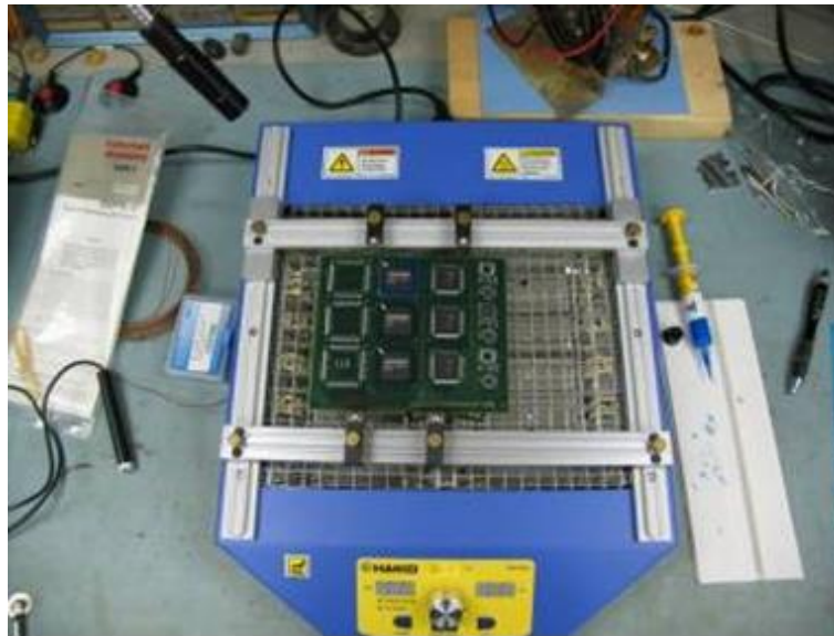
Figure 4- 14: Hakko FR-1012 preheater with sample test board.
