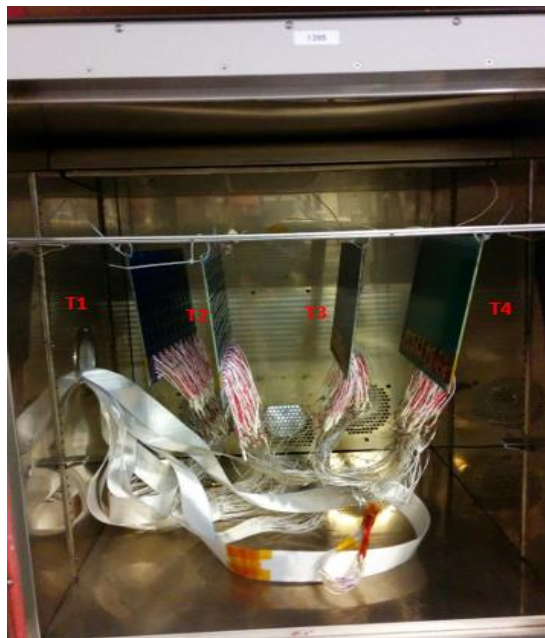
Figure 4- 4: Test board placed inside Sun thermal chamber with thermocouples.
