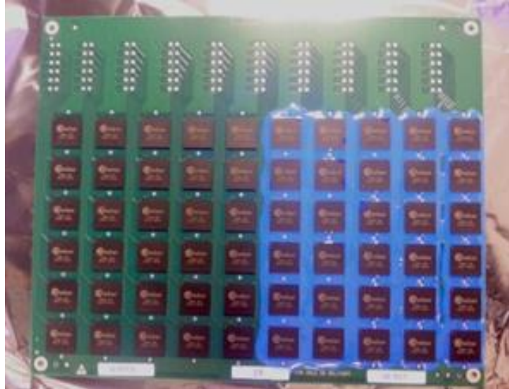
Figure 4- 1: Assembled test vehicle showing two halves of the board with one side applied with Thick conformal coating
