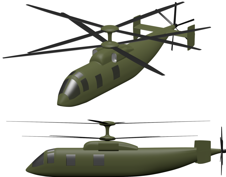
Figure B.1: Generic coaxial aircraft model (modified from original found in Ref. 132)
