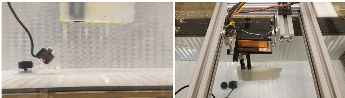
Figure 3.2: Experimental setup showing the viewing angle of the underwater camera and the suction cup mount used to attach it to the flow tank. The servo chassis and load cell array are shown mounted to a rigid beam with the airfoil attached to the control arm of the servo.
