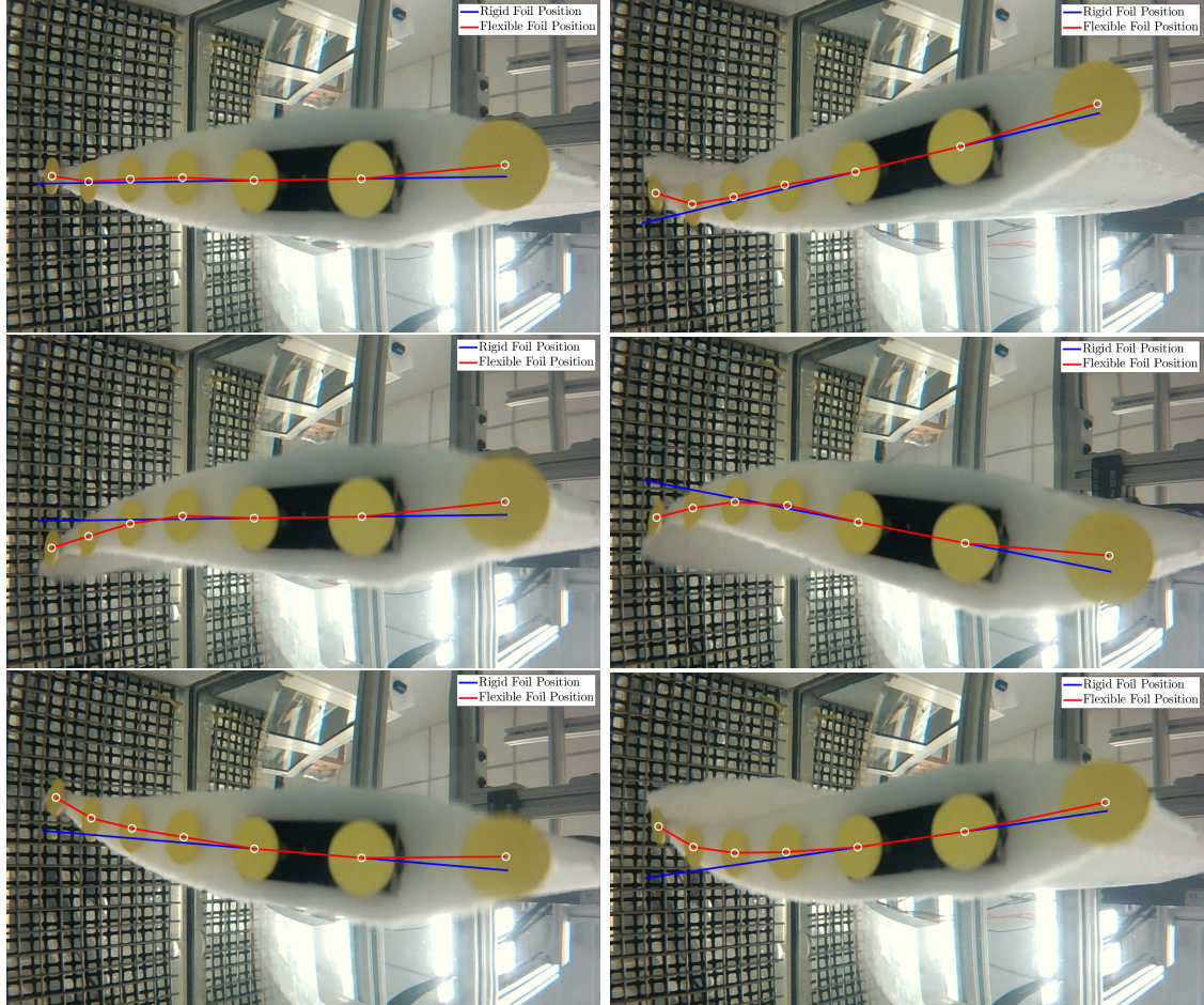
Figure 3.3: Sequential images of deformed flexible airfoil in water (read from left to right). The white circles show the position of the centroid of the markers, which are identified via computer vision. The red line shows the midline of the flexible airfoil. The blue line shows the overlay of the midline of a rigid foil at the same servo command angle.
