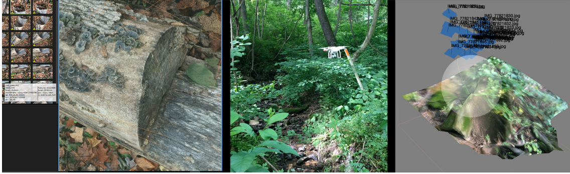
Figure 7.1: Trying to simulate realism using photogrammetry techniques. Left: A high-quality 3D mesh of a log I created by capturing several images of it. Middle: A drone I used to try to capture a large stream habitat. Right: A low-quality mesh created from the drone capture.
