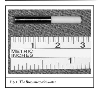
The Bion microstimulator's small size (27.5 mm x 3.2 mm) allows implantation adjacent to nerves via a less invasive technique than utilizing spinal cord stimulation technology. Previous studies have evaluated Bion implantation for pudendal nerve neuromodulation in the setting of refractory detrusor overactivity incontinence (14,15). At our institution, we have implanted 9 Bion microstimulators adjacent to the greater occipital nerve (GON) in an effort to treat refractory headache disorders.
