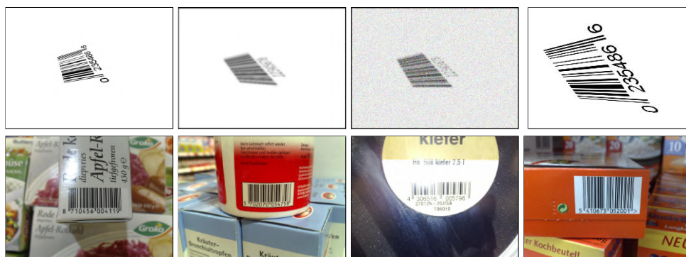
Figure 4.2: 1D barcode samples with different distortions, synthetic (top row) and real images (bottom row).
